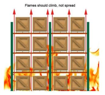
FM Global is more prescriptive with regards to transverse flue widths and horizontal spacing. To be effective as outlined above, flue spaces must be a minimum net width of 3 in. and ideally about 6 in. wide. A flue space's net width is a measure of its gross width minus any horizontal obstructions, such as rack uprights, located within the flue space.
